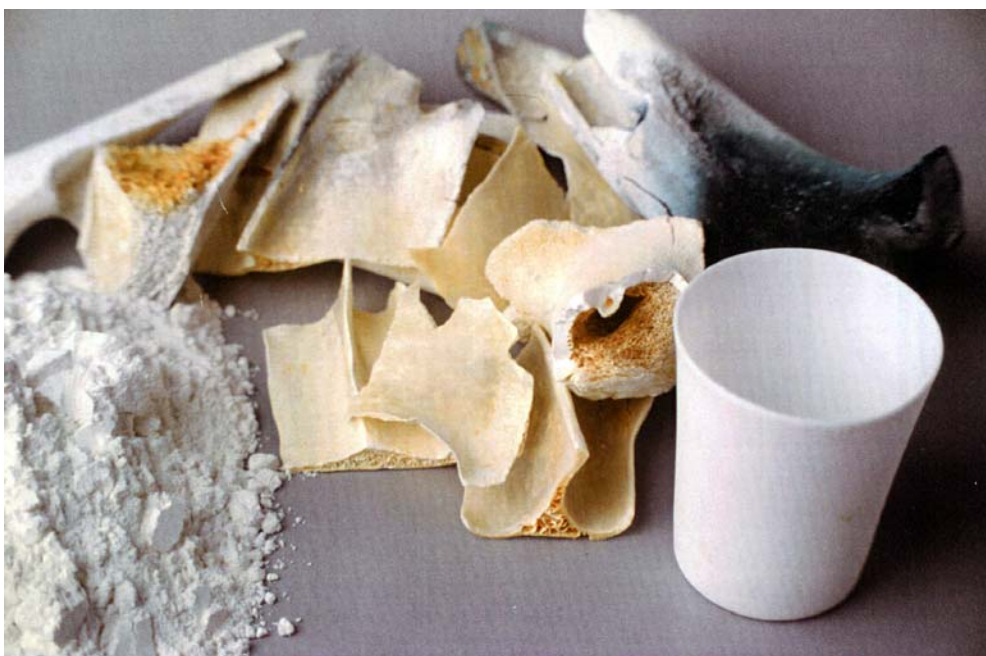
Fig. 1. The material process of reindeer bone china
