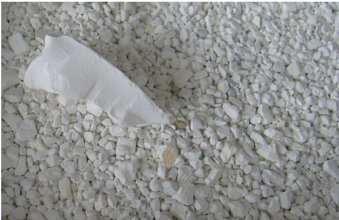
Fig. 2. Water grinded reindeer bone ash
