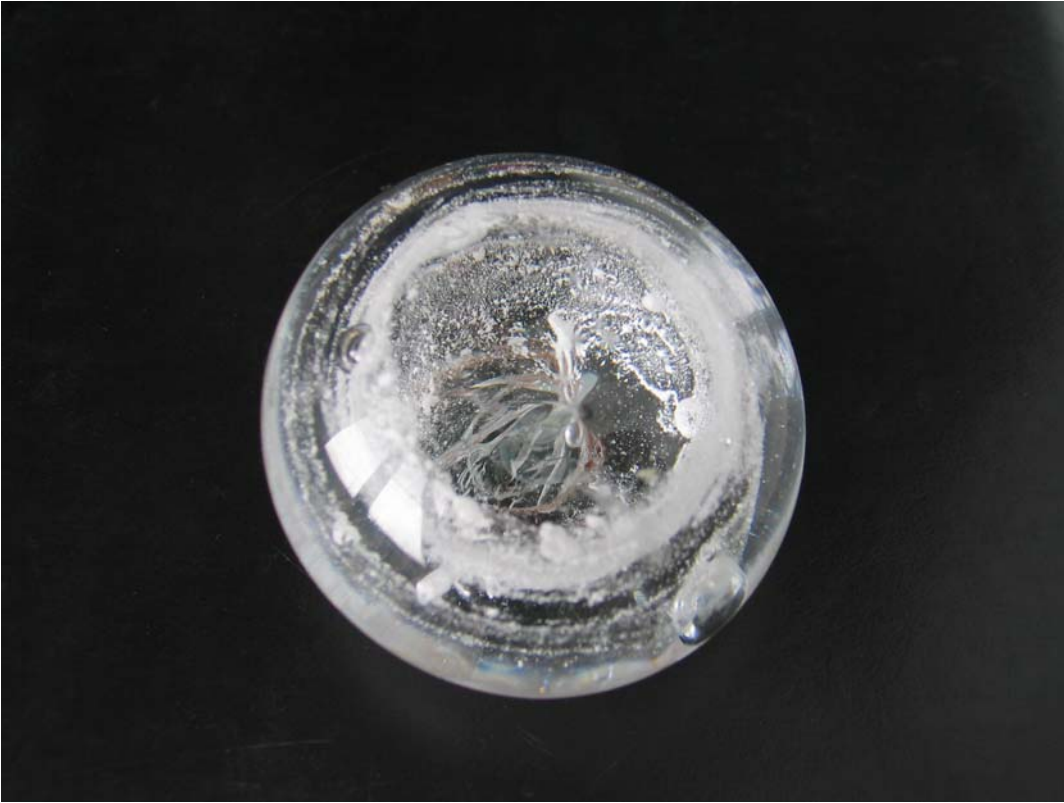
Fig.4. Opaque Reindeer bone ash baked in the glass material
