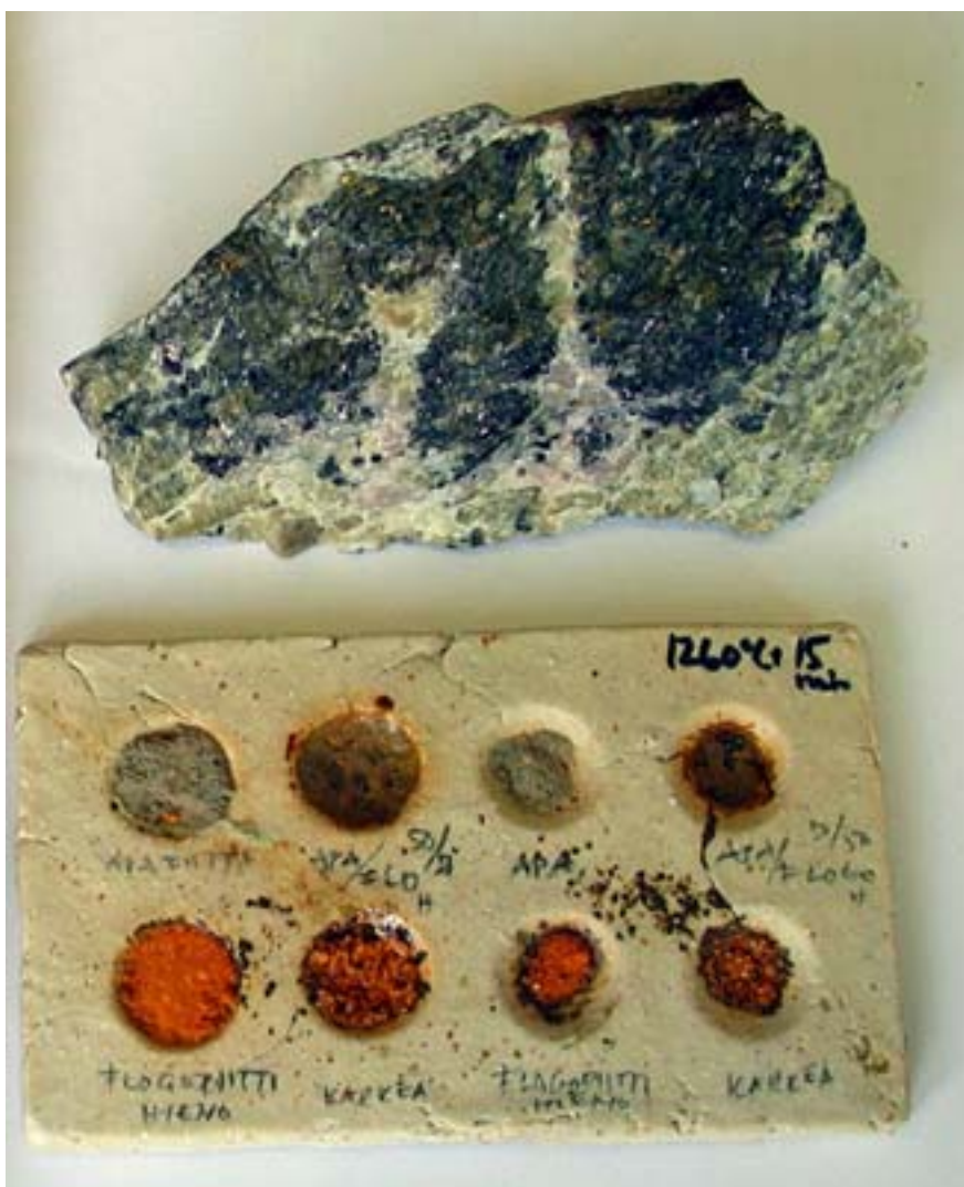
Fig. Apatite mineral (green colour) has 60% phlogopite mica (black colour). Test tile is fired 1260°C with 15 min soking time and colour of phlogopite mica turns brown red.
