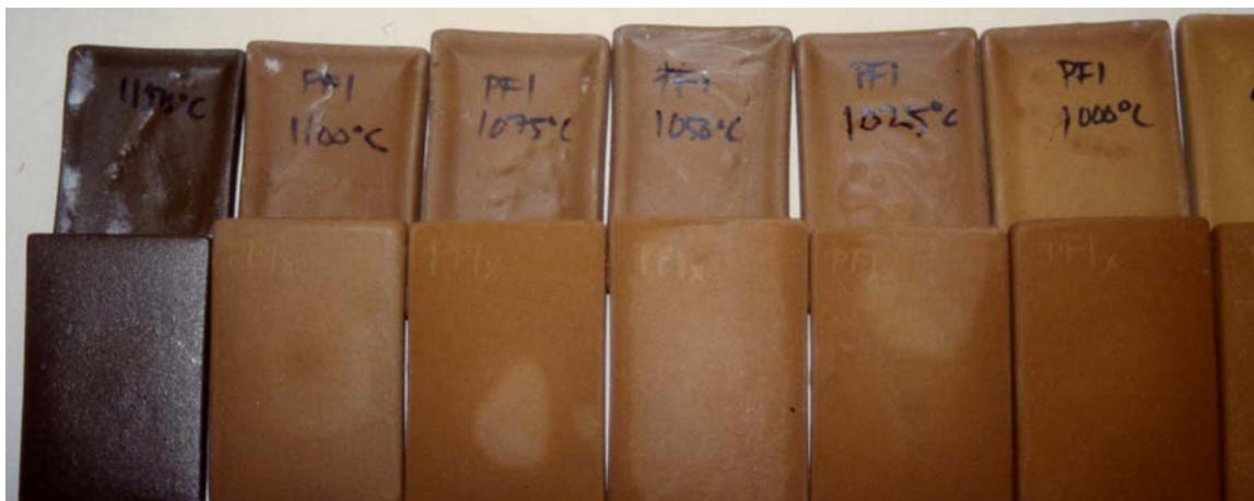
Fig. Test tiles PF1, 1150 - 950 °C, gradient of earthenware clay body
