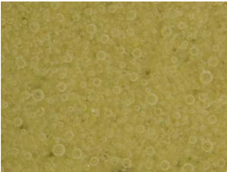
Fig.14b: Microscope enlargement 25.6. Hyplas 71 in engobe with Lime under clay color 10% wight. Lime color mixed with yellow and turquoise pigments. Test piece fired in the electric kiln 1200°C.
