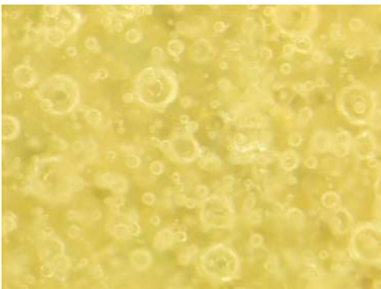
Fig.14c: Microscope enlargement 80. Hyplas 71 in engobe with Lime under clay color 5% wight. Lime color mixed with yellow and turquoise pigments. Test piece fired in the electric kiln 1200°C.
