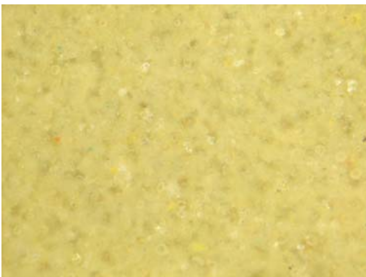
Fig.13c: Microscope enlargement 25.6. Hyplas 64 in engobe with Lime under clay color 5% wight. Lime color mixed with yellow and turquoise pigments. Test piece fired In the electric kiln 1200°C.
