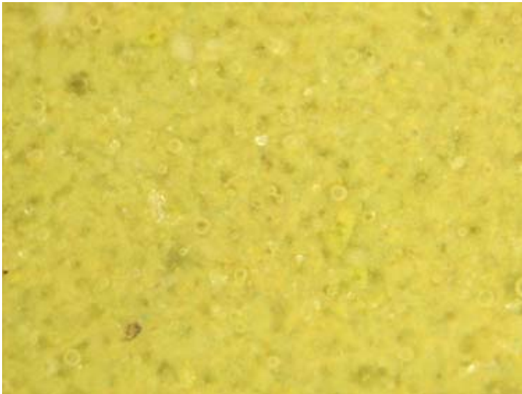
Fig.13d: Microscope enlargement 26.6. Hyplas 64 in engobe with Lime under clay color 10% wight. Lime color mixed with yellow and turquoise pigments. Test piece fired 1n the electric kiln 1200°C.
