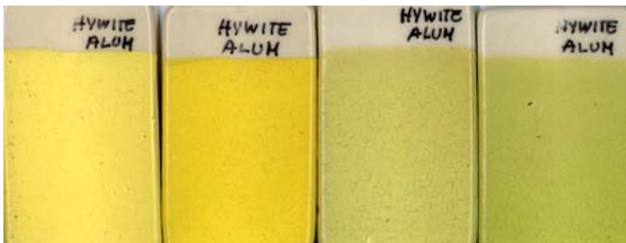
Fig.18: Ball clay Hywite Alum used in engobe with Citrus and Lime under clay color 5% weight and 10% weight.
