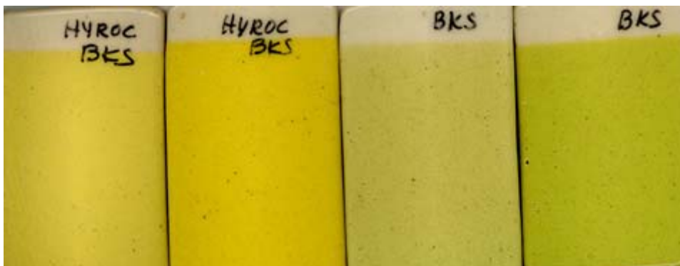
Fig. 12: Hyroc BKS in engobe with Citrus and Lime under clay color 5% wight and 10 % weight.
