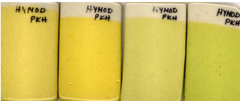
Fig.8: Hymod PKH ball clay used in engobe with Citrus and Lime under clay color 5% wight and 10 % weight.
