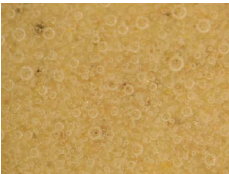
Fig.8a: Microscope enlargement 25.6. Hymod PKH in engobe with Citrus under clay color 5% wight. Test piece fired In the electric kiln 1200°C
