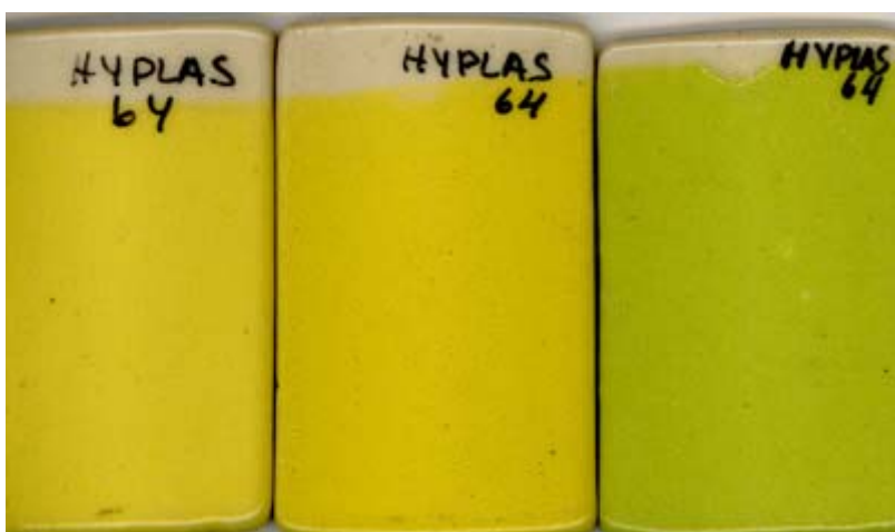
Fig.13: Hyplas 64 in engobe with Citrus and Lime under clay color 5% wight and 10 % weight.
