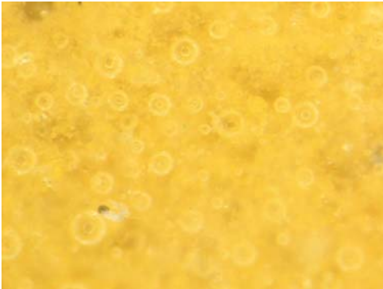
Fig.7b: Microscope enlargement 80. Hymod At in engobe with Citrus under clay color 10% wight. Test piece fired In the electric kiln 1200°C.
