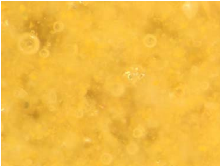
Fig.13b: Microscope enlargement 80 Hyplas 64 in engobe with Citrus under clay color 10% wight. Test piece fired In the electric kiln 1200°C.
